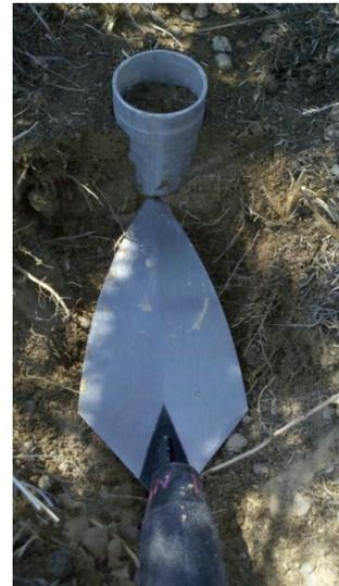
use the metal spatula to evenly distribute and *lightly* pack the material. The base of the core is your contact surface for the soil moisture retention measurements so a flat continuous surface is important (see adjacent picture). You can add several drops of water to the base of the core to adhere the added soil material.
